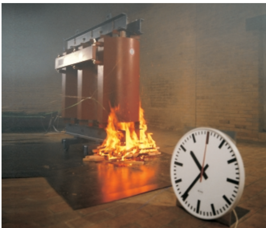
Fig. 51: Flammability test of cast-resin transformer
